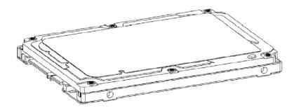
Figure 1-5 2.5-inch HDD
